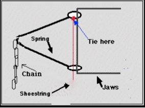
Then, stand on the trapchain, pinning the trap to the ground and haul up on the shoestring This will compress the spring. Pull and take up the shoestring until both sides of the spring meet. Tie off the shoestring and repeat
