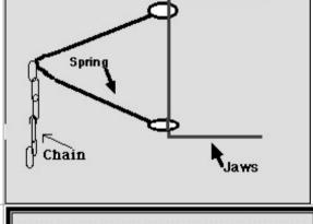
To release the trap, tie one end of a shoestring to the top loop of the spring where it runs along the jaws, run the shoestring through the bottom spring loop and then back through the top spring loop.
